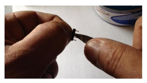
4 pin  $(2\times2\times.1")$  Molex dual row header cut in half and inserted.
