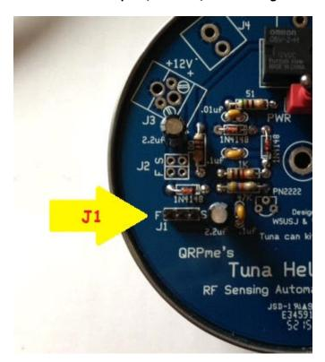
J2 is 2 seperate sets of 2 pins. Gently cut the 4 pin  $(2\times2\times.1")$  Molex dual row header in half.
