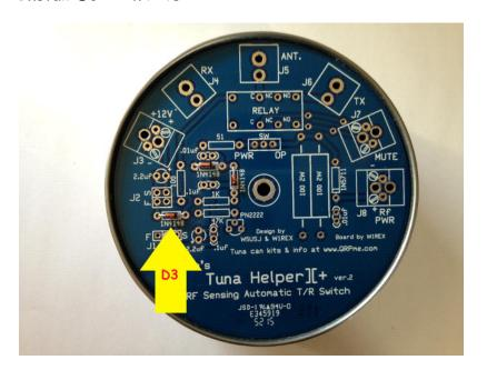
Spread the leads slightly and turn over the PCB
