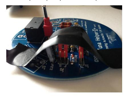
Turn the PCB over and solder SW , Relay , J1 and J2 pins.
