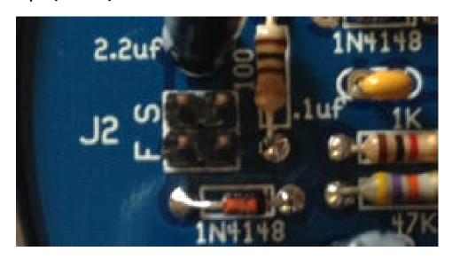
Place the Headers on J1 and J2. \*\*\* This is so to aid in securing the pins in place while you place a piece of tape on them so they will not fall out when you are soldering them \*\*\*
